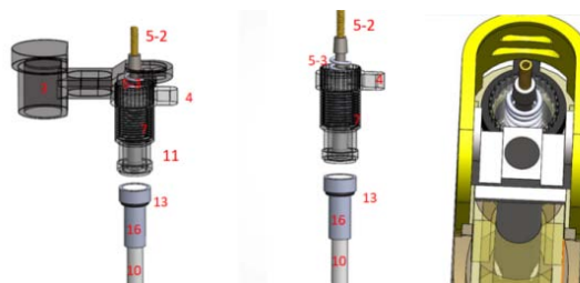
Figure 4. Schematic diagram of fire power maintenance (left) with buttons (middle) fire power adjustment part (right) with windscreen.
